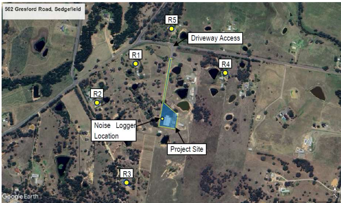
Figure 3 - Receivers tested – From the Noise Assessment by Spectrum Acoustics (232350-10212), dated February 2024
