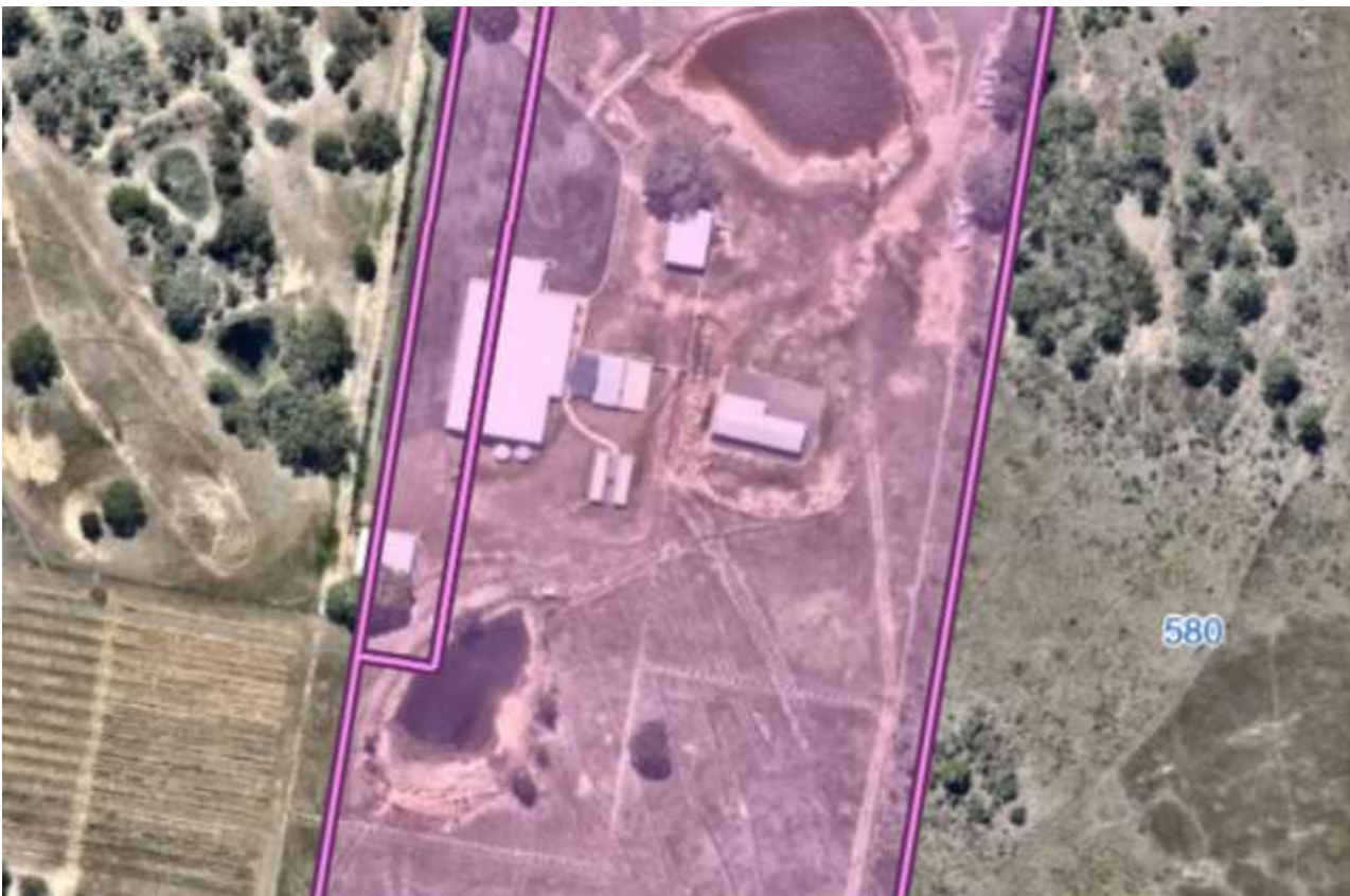
Figure 2 – Development Location – Note the cadastral map does not correctly line with the aerial imagery due to parallax errors on rural imagery.
